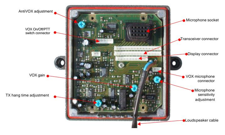
The VOX/Junction Box normally comes factory-adjusted for typical in-vehicle use so it will not be necessary to tweak the microphone sensitivity and transmitter hang time presets on the board. To avoid the VOX being erroneously triggered by received signals, fit the small condenser microphone as far away as possible from the loudspeaker. The AntiVOX circuit will attempt to cancel loudspeaker sounds.
